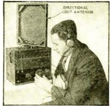
Fig. A. The loop points toward the station.
