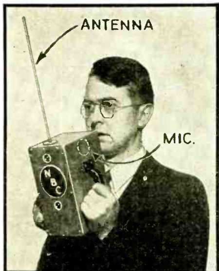
Fig. D. NBC's "beer mug" for table transmitter.
