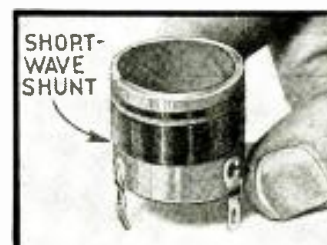
An "add-on" S.W. coil unit. (1120)
