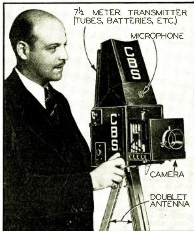
Fig. B. The "photo-mike," and its creator, E. K. Cohan, of CBS.
